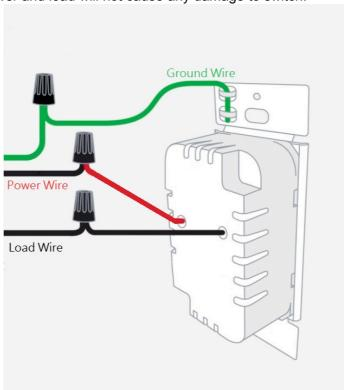
Step 4: Mount switch into the wall. Screw in the snap plate and push the plate onto it.
